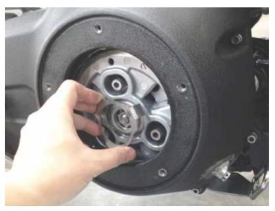
6.Install the VP Clutch. Use the provided bolts and tighten evenly with 5mm Allen wrench. Finally, tighten to a torque of 7.5-9.2 ft-lbs (10.2-12.4Nm).
