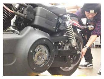
3. Rotate the rear wheel until we could align the clutch studs bolts horizontally at the bottom to the ground.
