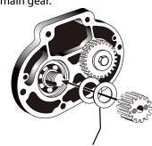
Adjust the holes with the shims.
