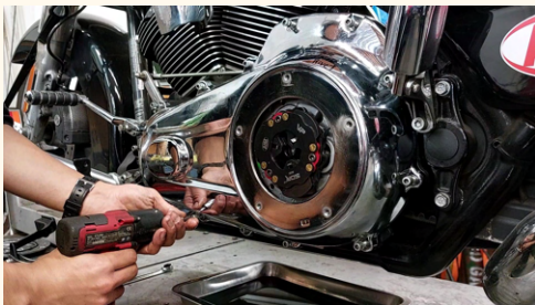
27. Tighten bolts with drill and then wrench for final tightening.
