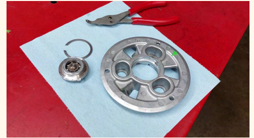
7. Remove retaining ring and previous clutch adapter.
