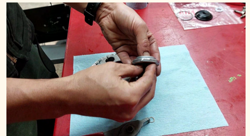
14. Remove small c-clip and release rod from previous adapter and place into new adapter.
