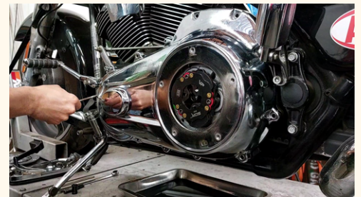
26. Put bolts back on by hand to avoid cross-threading.
