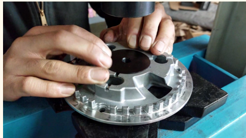
9. Place a part like an aluminum cylinder on top of the adapter.
