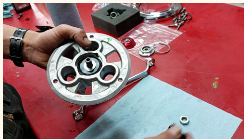
13. Place adjusting nut and flat washer (comes with the kit).
