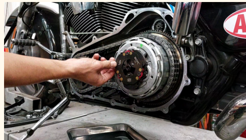
22. *Check movement of SDR Max V2 fly weight flaps.
