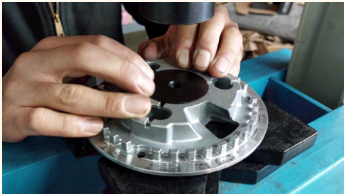
8. Place pressure plate / cable clutch adapter on hydraulic press flat surface.
