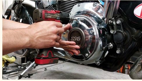
31. Tighten bolts with drill.
