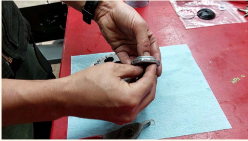
15. Adjust small c-clip left to right to see if it's seated. If movement is rough, it's not seated correctly.
