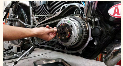
20. *Check movement of SDR Max V2 fly weight flaps.
