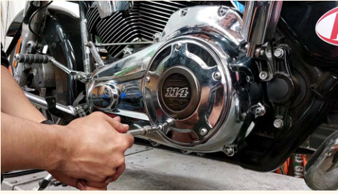
30. Final tightening with wrench
