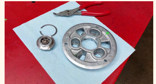
7. Remove retaining ring and previous clutch adapter.
