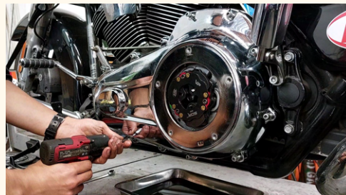
25. Tighten bolts with drill and then wrench for final tightening.
