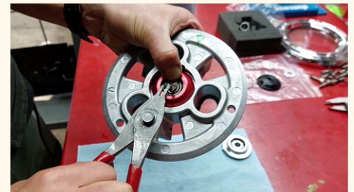
14. Adjust small c-clip left to right to see if it's seated. If movement is rough, it's not seated correctly.
