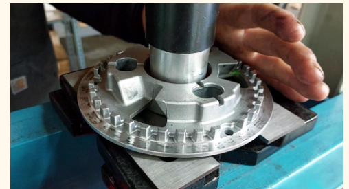
10. Use hydraulic press to push adapter into pressure plate.
