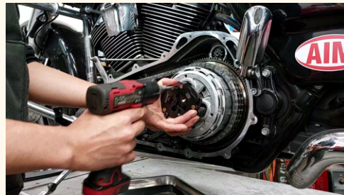
6. *Remove SDR Max V2 bolts evenly, remove springs and pressure plate.
