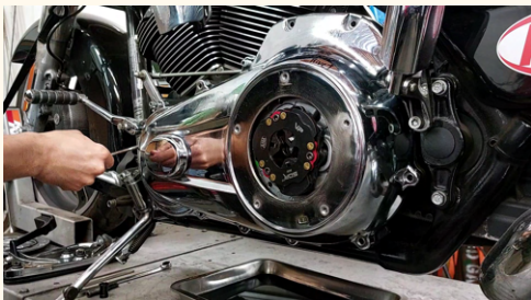
24. Put bolts back on by hand to avoid cross-threading.
