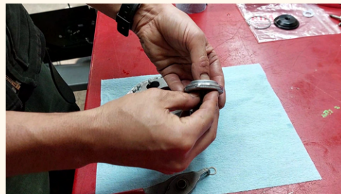
13. Remove small c-clip and release rod from previous adapter and place into new adapter.
