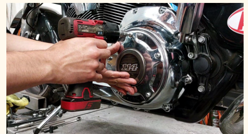
29. Tighten bolts with drill.
