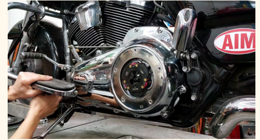
3. (Varied by model) Remove any additional parts on primary cover.
