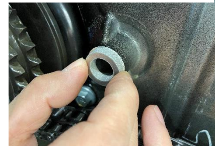
Mid control bikes are required to install small ¼" spacer onto the shift linkage. Without this spacer and gasket, there will be a potential leak from the primary.
