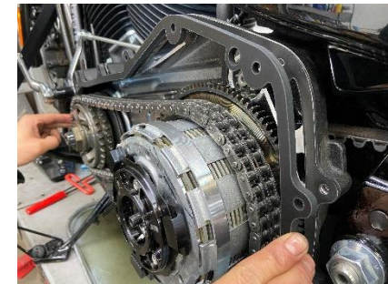
Install the primary gasket first then the primary spacers followed up by another gasket.
