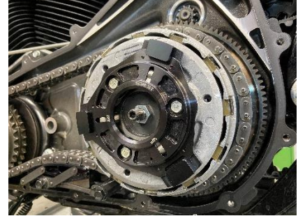
How the SDR ST High Performance version looks like when installed on the clutch system.
