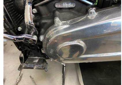
Step 3: Remove foot board / peg for easier access to the primary cover.
