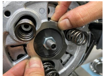
Here is a perfect time to install the wear shim and replacement springs if necessary.
