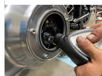
Torque all necessary bolts and fill the primary with proper fluids. Please refer to your owner's manual for proper fill procedures.
