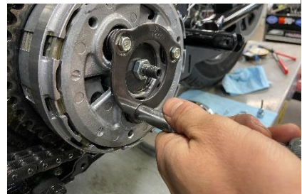
Step 6: Loosen and remove the 3 10mm bolts holding the retaining plate.
