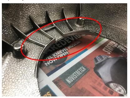
3. Circled in red, portion will need to be grinded will be right below the bottom of the derby cover opening.
