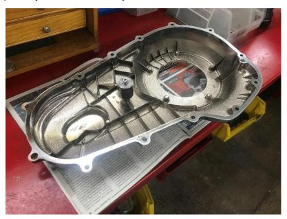
2. Remove the primary cover and make sure to clean of an excess oil.
