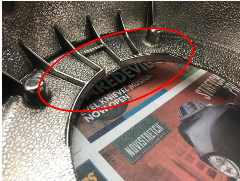
3. Circled in red, portion will need to be grinded will be right below the bottom of the derby cover opening.
