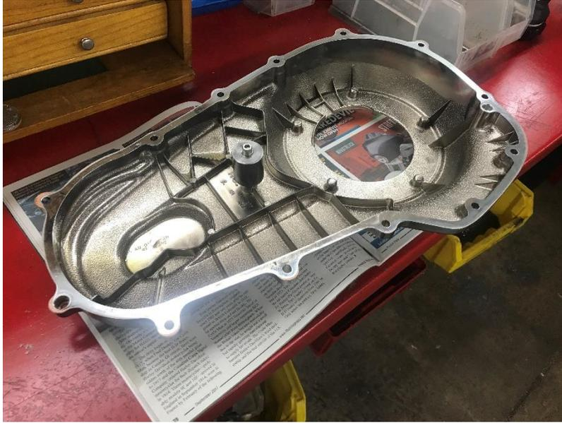
2. Remove the primary cover and make sure to clean of an excess oil.
