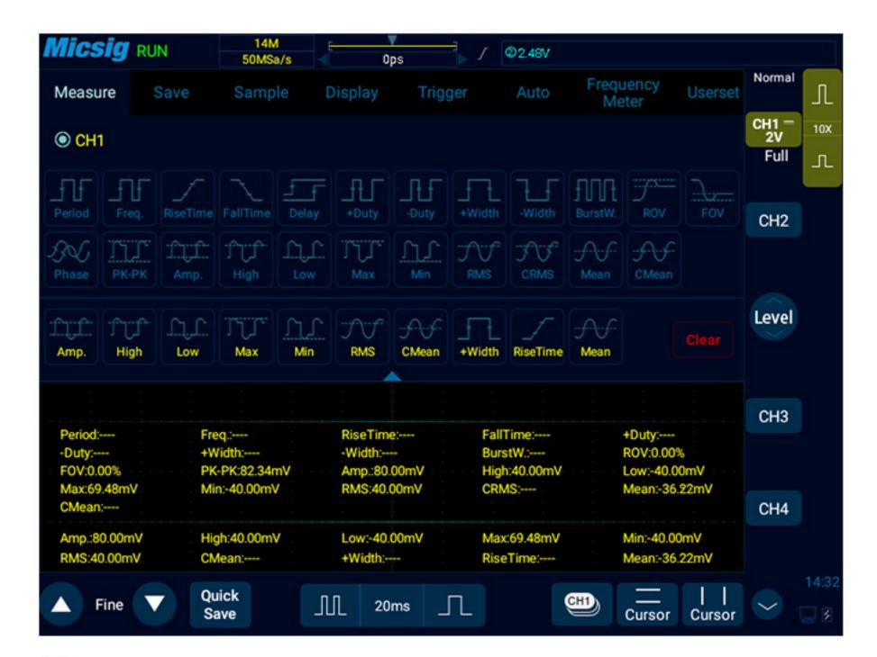
31 automatic measurements. Various automatic measurements can meet different measurement demand. It can be display all in one page.
