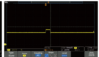
D/D Converter Surge Testing
