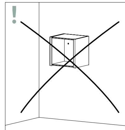
Modules must never be mounted freely suspended. The wall mounting serves only to secure against tipping over.
