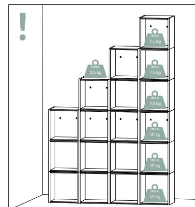
Maximum load capacity is 10 kg per module on the lower three rows of shelves and 7.5 kg from the fourth to the sixth row. The maximum load capacity on the upper surface of the module is 2.5 kg. Please always store heavy items in the lower modules. Be careful not to overload the outside edge of the shelf.
