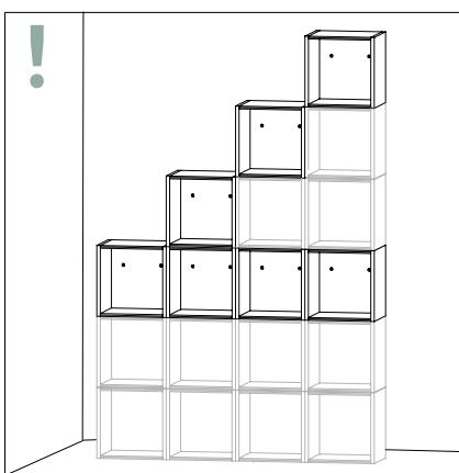
From a height of 3 modules, the uppermost module must be fixed with the enclosed wall bracket. From the fourth on: Always use two wall brackets (3rd module and top module). The maximum permissible stacking height is six modules.
