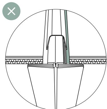
In order to place the connector correctly, you must press the layer with the visible longitudinal shaft slightly outwards. The spatula helps you here.
