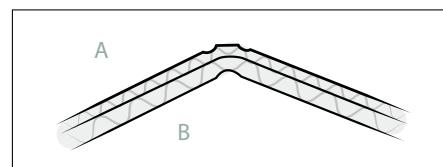
**PLEASE NOTE:** Corrugated board has two sides. The side with the smaller flutes should always be on the outerside. The side with the larger flutes is inside.
