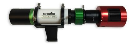
For other telescopes, the EvoFF can fit into any 1.25" focuser or into a 2" focuser using a standard 1.25" step down ring.
