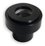
To get the best image quality, the backfocus distance from the field flattener to the image sensor must be set correctly. For the EvoGuide 50ED, the required distance from the male T-threads on the camera side of the flattener is 34mm. For other focal length telescopes, see the table below.
