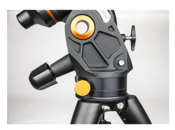
When setting the mount head and Landing Pad onto the tripod, you can simply let the Landing Pad sit against the top of the tripod, then rotate the mount until the pan-head screw drops into place in the hole. This makes guiding the mount into place easy.
