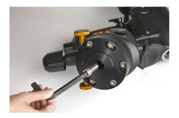
Use the large hex wrench to install the M12 bolt into the bottom of the Landing Pad. Make sure this bolt is tight. You can tighten the M8 bolts now as well. If the Landing Pad is rotated too far one way, one of the bolts may not reach, so be sure the rectangular block the bolts lock onto is centered.
