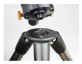
There is a small pan-head bolt in the bottom of the Landing Pad that helps guide it into one of the (now empty) post holes on the top of the tripod. It should go into the hole that is away from one tripod leg, which will be to the south (in the Northern Hemisphere). This places the orange adjustment knobs to the south, away from one tripod leg.
