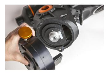
The easiest way to attach the Landing Pad is to lay the CGEM mount head on its side. The post on the bottom of the mount head will insert into the matching cutout in the top of the Landing Pad. The rectangular block on the top of the Landing Pad should fit between the M8 screws you installed in place of the original adjustment knobs. Hold the Landing Pad flat against the base of the mount head and snug the M8 screws by hand to help hold it in place.
