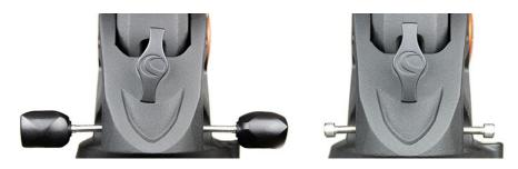
Remove the two azimuth adjustment knobs from the mount head. These are not used with the Landing Pad, and are replaced with fixed bolts to avoid the possibility of grabbing the wrong adjustment knobs in the dark.
