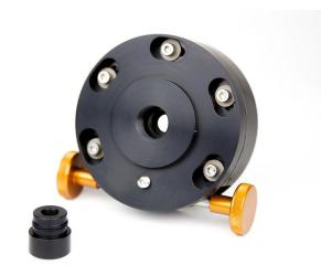
Unthread the cylindrical mounting post from the bottom of the Landing Pad. There is a set screw that can lock this post in place, and it should be loose when the Landing Pad is new, but if the post will not unthread easily, check this set screw.
