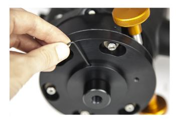
Once in place, use the small hex wrench to lock down the set screw that holds the mounting post in place.
