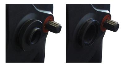
**Above**: Removing the smaller SCT threads from an 11" SCT to expose the larger mounting threads
