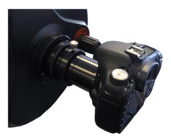
The SCT Corrector has a 2" diameter body, allowing it to fit into a 2" visual back or 2" focuser drawtube. Ideally, the SCT Corrector will be mounted as close to the back of the telescope as possible. The performance of the lens does not change significantly if the SCT Corrector is farther from the telescope, but the focal reduction factor changes, reducing the field of view and increasing the telescope's focal ratio.
