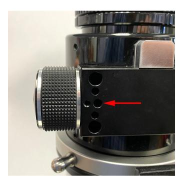
Remove the focus knob from the left side of the Esprit focuser. There is a set screw on the knob that is accessible through the center hole on the left side of the focuser pinion block. You will need to rotate the knob to line up the screw with the hole. The 2mm hex wrench included with the EAF motor will fit this screw.
