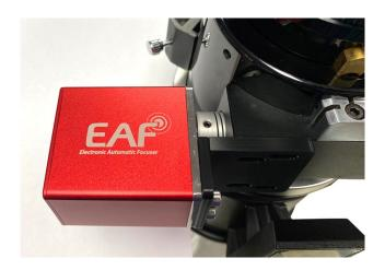
Insert the shaft on the motor into the shaft coupler. Slide it far enough in so that the necessary slots on the bracket line up with the mounting holes on the focuser. The Esprit 80 uses the narrower pair of slots, the larger Esprits use the wider pair of slots. Once in place, tighten the two set screws on the shaft collar to the motor shaft.
