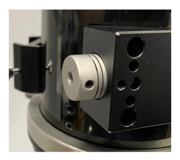
Install the appropriate shaft coupler (included with the EAF) onto the shaft where the knob was. You access the set screws through the same hole used to remove the focus knob.
