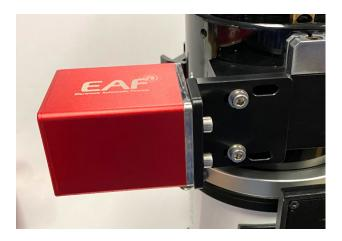
Use the screws included with the bracket to attach the bracket to the focuser. The Esprit 80 uses the longer screws, the larger Esprits use the shorter screws. The image above shows the installation on the Esprit 80. The image below shows an Esprit 100 (same as 120/150).
