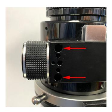
The EAF bracket attaches to the existing mounting screw holes on the left side of the Esprit focuser. Start by removing the screws from these holes. The 3mm hex wrench included with the EAF motor will fit these screws. The screws that come with the bracket will be used to replace these screws after the bracket is installed.
