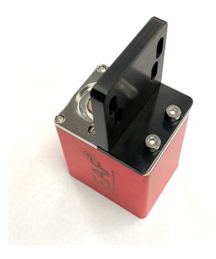
Use two of the screws that come with the EAF kit to attach the bracket to the motor. The long plate on the motor goes toward the shaft on the motor. The bottom edge of the short plate should be aligned with the bottom edge of the motor housing, but there is some room for adjustment if necessary.
