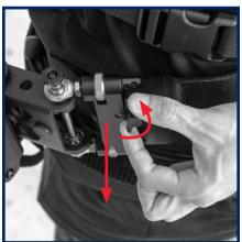
If the rig tends to move straight **towards** you; loosen the top thumbscrew slowly, until the rig behaves, and then tighten the bottom thumbscrew.
