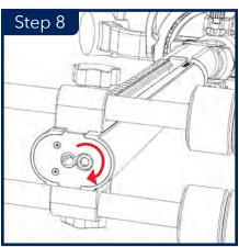
Attach the post to the handle by turning the retaining screw clockwise with the provided 5mm hex wrench.
