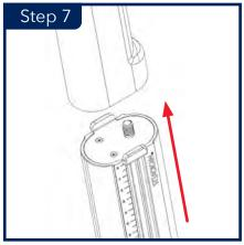
Align the Steadimate-RS post with the bottom of the handle, taking care to place the retaining screw at the 1/4"-20 hole near the FRONT of the handle.
