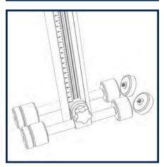
To make large adjustments to the tilt feel, we'll remove pairs of weights and compare how it feels to tilt with less counterweight.
