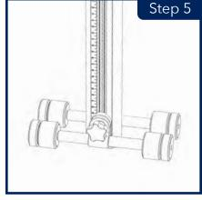
Remove the factory tripod base from the bottom of your stabilizer handle and set it aside.
