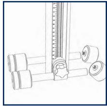
Redistribute the two small weights from the front of the rods to the rear, then re-balance by sliding the rods fore-aft.
