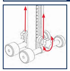
Now fine tune the tilt feel by raising the weight rods a little at a time, and testing, until you achieve fingertip control of tilt.
