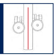
Continue sliding the weights higher on the post until the effort required to tilt the stabilizer is minimized.
