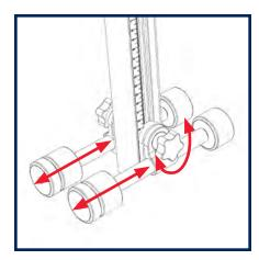
If the tilt remains bottom heavy, repeat the previous steps, this time remove the large weights at the rear of the rods.
