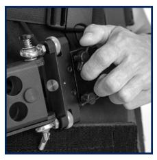
Secure the arm to the vest by tightening both fore-aft adjustment knobs equally, so the sockets are parallel.
