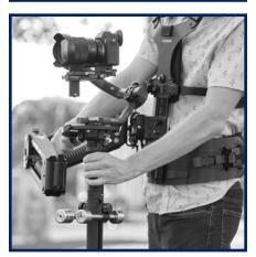
Repeat the arm adjustments as needed until the Steadimate-RS system is neutral when sitting slightly to your operating side, in balance with your vest.
