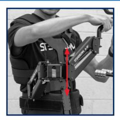
If the arm is lifting too much, or too little, adjust the lift knob on each arm section until both sections of the arm are neutral just above horizontal.
