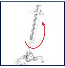
Continue removing weight pairs, re-balancing fore-aft, and testing, until the system will not rest with the camera at the top.
