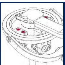
NOTE: The four screws on top of the pan bearing that secure the NATO mounts MAY need to be loosened slightly to help properly align the mounts to the DJI Ronin RSA/NATO ports, then re-tightened.
