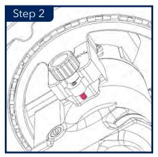
Ensure the thumb screws are out of the way, so the RSA/NATO ports fully seat into the NATO mounts.
