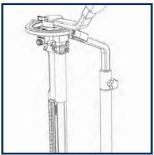
Use a C-stand or a heavy-duty light stand, with the included adapter, to support the system while balancing.
