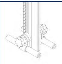
**NOTE:** for lightweight cameras, you may be able to remove ALL of the weights without the post inverting.
