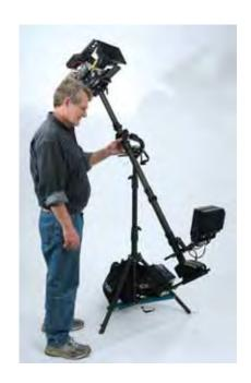
The operator dynamically balances a long sled using the same procedures as with a shorter sled. The trial and error method is fairly quick. However, because there are so many possible configurations with the Ultra<sup>2®</sup>, or similar Steadicam® rigs, spin balancing for each one can be time consuming and unproductive. Use the Ultra<sup>2®</sup> Dynamic Balance Spreadsheet to virtually discover how to get your rig into dynamic balance under various conditions.
