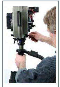
Tip: To speed up the balancing process, hold the sled vertical with your operating hand on the gimbal. Hold the gimbal the same way you would do while operating. Hold the sled absolutely vertical as you adjust the side to side or fore-aft balance. Turn the adjustment knobs with your other hand (or use the remote) until you feel no pressure on your operating hand, and the sled will be in static balance.
