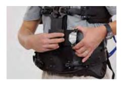
On the arm, pull the "parachute pin," flip the mating block, and reinsert the parachute pin with the kick back link rotated (see page 6). Note that the mating block is now reversed; the upper side to side adjusting screw is now the lower screw and vice versa.
