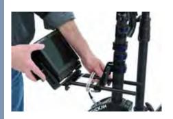
Lower the monitor and/or extend the posts to balance a heavy camera, gain lens height, and/or to increase tilt and roll inertia (or all three!!).
