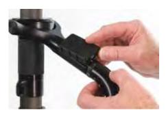
When returning the remote to the handle, insert the pins carefully and do not force anything.
