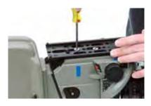
If possible, attach a second dovetail plate to the top of the camera, directly above the other dovetail. This may require additional hardware, such as a special low mode bracket for your camera.
