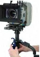
A small warning: do not over-tighten the caps against the bearings, as this will cause binding. Just tighten each cap down to touch the bearing. If the bearing starts to bind, just back off one of the two end caps until the gimbal is free again. The blue whale tool also makes it easy to take apart and clean the gimbal if this ever becomes necessary.
