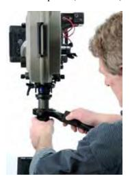
Trim side to side with the camera, using the knobs on the stage. If your rig is equipped with the stage motor remote control, you can use it as shown. Fine tune fore-aft balance with the motors as well. Double check that the post is perfectly vertical. Give the sled several careful test spins. Very important: do not spin the rig very fast – certainly not any faster than your usual panning speed.
