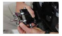
Use a 1/4" allen to adjust the "side to side" screws. When wearing the rig, be sure to hold the centerpost in line with the "in-out" thumbscrews. This will take the loading off the side to side screws.
