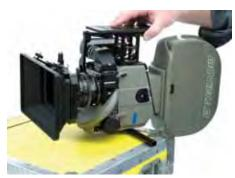
Finding the camera's fore-aft center of gravity.
