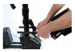
The stiffening system is very useful with normal length sleds when the shot has violent moves or high stresses, such as during a vehicle shot on rough roads.
