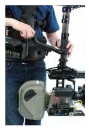
The F-bracket brings the arm back into a proper relationship with the inverted sled. Without an F-bracket, the end of the arm will be next to the camera. Switches are impossible and operating is severely limited.
