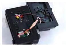
Normally, the red stripe wire is connected to the other red stripe wire (for 24 volts and 14 volts via the converter or 12 volts via the rear battery). Carefully pull apart the connectors, and pull out the solid red wire. Connect the solid red wire to the red stripe wire. This will connect the two batteries in parallel and disconnect the converter from the circuit. 24 volts is not possible with only two batteries in this mode.
