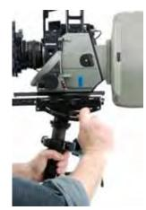
Note: Don't grab the stage by the nosebox to adjust tilt. Be sure to loosen the arc clamps fully and grab the camera or dovetail plate. Don't force anything; it should move fairly easily.
