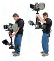
Note that the operator can reach higher with his operating hand, but the arm can't reach any higher. Do this with the arm attached to the socket block at its lowest practical point on the vest, and with the shortest possible arm post. This will generate your primary range of gimbal heights. You may find it useful to have someone measure this range of lens heights.
