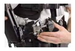
The G-70x<sup>™</sup> arm socket is inserted into the socket block on the vest.
