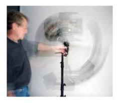
Now let the sled rotate (drop) through vertical and note the time. A two second drop time is a good starting point. 2 to 4 seconds is typical. Raise or lower the gimbal slightly to get a faster or slower drop time. (Again, only release the gimbal clamp when the rig is horizontal!!) A different drop time is required for long mode shooting.
