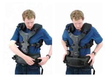
**Push the vest down on your shoulders again,** be sure the spar is vertical, then snug up the hip pads. If the hip pads are tightened first, the vest will tend to ride high until loaded, and then it will slip around under load.
