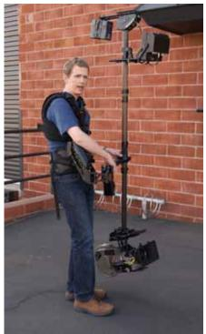
We typically use the F-bracket to bring the arm back into a proper relationship with the sled so we can pan, tilt, and make switches without hitting the camera. A longer post from the F-bracket to the gimbal is impractical. Even with the shortest possible post, one cannot reach the gimbal at the bottom of the G-70<sup>™</sup> arm's range. A longer post only lowers the maximum height you can reach.
