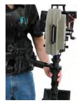
We can use the F-bracket in high mode to lower the range of lens heights. It's sometimes called "low high mode." How low we go is often a function of how low we can reach.
