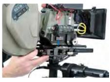
Push the locking lever forward to fully lock the camera into place. You are now ready to static balance the sled.
