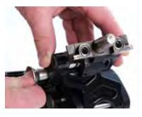
To set your threads, first dial the lower side to side screw all the way in, then adjust the upper screw to your threads - about 2 to 2.5 turns out. Use the same procedure to change back to left side operating.
