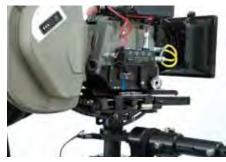
Dovetail locking lever fully open.
