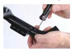
Orient the remote by screwing the curved handle in or out. If the handle is too far in, you can't easily remove the remote via the black knurled ring, and you might have to back the handle off one full turn. Loosening the setscrew a lot further and unscrewing the handle is also how you access the "tilt" bearings and shaft for cleaning.
