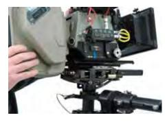
Place the camera above the camera mounting platform. Be sure the locking lever is fully open. Angle the left edge of the dovetail into the holder. Be sure to keep everything parallel. Lower the right side into the holder.
