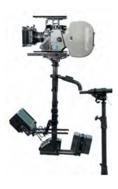
With the camera and monitor set, release the two battery rod clamps and pull out the battery until the sled balances upright. Balance as best you can with the battery – do not move the camera or monitor – then tighten the battery rod clamps.
