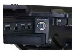
•Port side: +14VDC and video out. 4 pin HRS.
