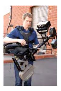
Cautionary Tip: When in low mode and grossly adjusting the camera position by sliding the dovetail, be sure to: 1) support the camera; and 2) lock the dovetail by pushing the lever forward. Balance as you would for high mode.
