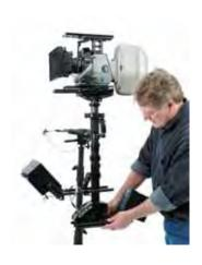
Next, static balance with the battery so the sled hangs perfectly vertical fore-aft. Use a slow drop time (3-4 seconds).
