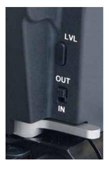
Pushing the button (LVL) for less than 1 second will reset the sled level (sets the "zero offset").
