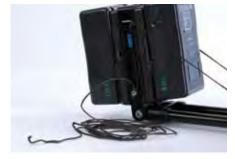
The Vectran® line is given its final tension by extending the telescoping posts slightly, pulling out the monitor rods as shown, and/or by tilting the sled horizontal with the monitor down and retightening the line.
