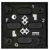
The four buttons on the frameline generator control the framelines, crosshairs, on-screen horizon position, and battery indicator position, as well as the frameline style, crosshair style, graphic brightness, graphic elements on or off, and two stored frameline and graphic presets.
