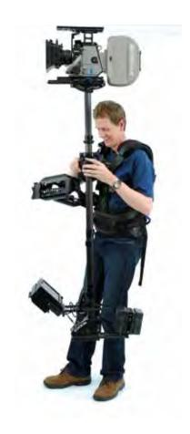
Instead of using a drop test, tilt the sled with your operating hand and note how much force is required. Compare this force to your normal length sled's feel. Accelerate the rig and note the pendular action. Again, adjust the bottom heaviness accordingly, depending on the requirements of the shot.
