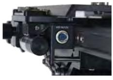
•Starboard side:+12VDC (regulated) and video in. 4 pin HRS.
