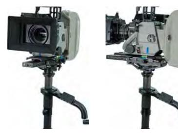
• Balance side to side and fore-aft as precisely as you can to get the post vertical. We recommend you use a bubble level on the stage, and be sure that the tilting head is set 90° to the post (horizontal). Rotate the sled 90° so that the camera is aimed at along the axis of the yoke handle, as shown in the right photo, above. Tweak the fore-aft balance as precisely as you can, then do not touch the stage adjustments for the rest of the procedure.
