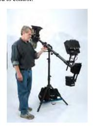
The uselfulness of any long mode sled is greatly enhanced by the addition of an integral tilt head and a motorized stage, if so equipped. Use the tilt head to keep the rig more vertical, reducing the spatial translations, and, at the same time, reducing clearance problems between the sled and objects on the set.
