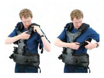
The chest pads are snugged up next. You should be able to breathe a little, but the vest should not be able to slip forward and down. Diaphragmatic breathing (like a baby) works best.
