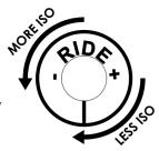
To adjust the arm for maximum iso-elasticity at any given lift, we turn the Ride knob counterclockwise until the arm segment begins to "lock" up or down at the extremes of travel. We then turn the ride knob clockwise a couple of turns. This will keep the arm from locking up or down. We test and micro-adjust the lift and ride knobs as necessary.
