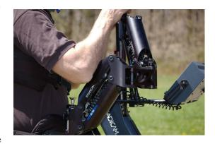
Lift can be altered by forcefully holding the arm segments at the correct angle while adjusting, but be prepared for some exertion! You might be shocked how energetic the springs feel if you are raising or lowering the lift by 30 pounds (13.6 kg)!
