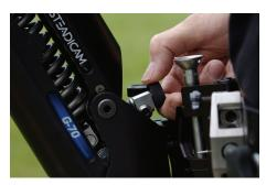
Adjusting the ride: the arm must be angled up at the top of its range.
