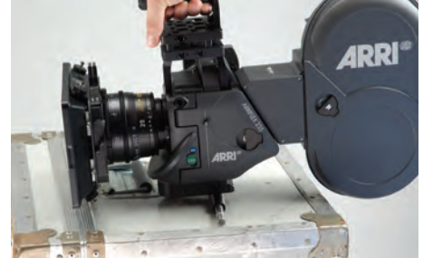
Finding the camera's fore-aft center of gravity.
