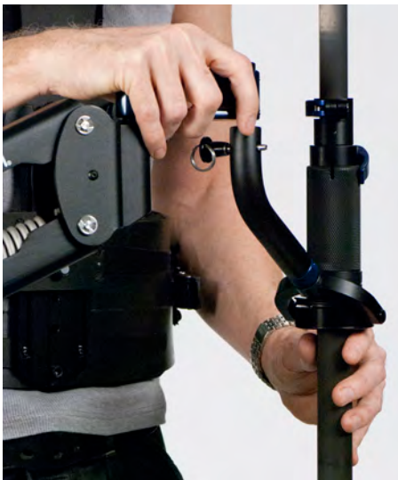
Hand positions for operating with the F-bracket.
