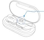
By using the Setting Button on the Charging Case, you can check the battery status of the Charging Case and reset the Hearing Aids to factory settings.
