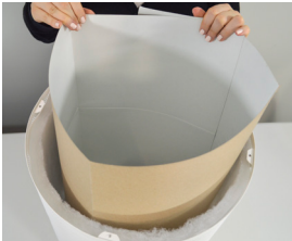
4. Insert the tube into the filter chamber inside the prefilter, opening the top of the spiral to make a slight funnel.
