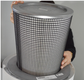
7. Replace the HEPA filter that had been set aside.
