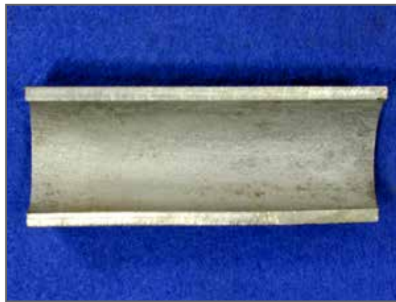
New Steel FPS Pipe Treated with MICtreat® FPS Chemical
