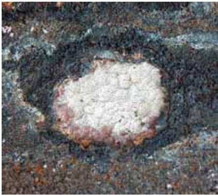
Figure 3 — Under-deposit pitting corrosion showing distinct pits within pits, characteristic of MIC.
