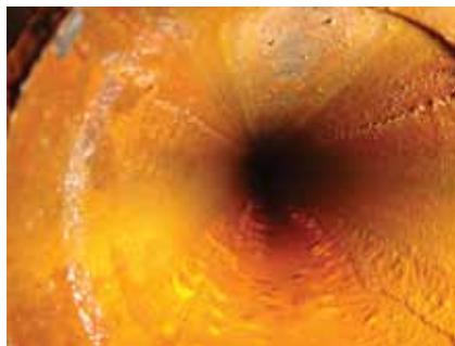
*Figure 2 – Mid-stage MIC, black pipe in wet FPS*
