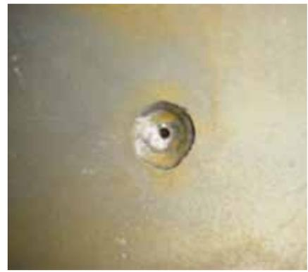
Figure 5 — Pinhole leak in dry galvanized FPS pipe. This pitting occurred under discrete deposits located where water puddles had been.
