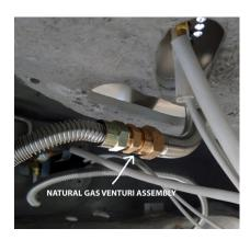
4 - Install the propane venturi assembly (NOTE: Use gas tape on the burner pipe thread, not the fitting between the venturi assembly and the stainless steel flex pipe) and reattach the stainless steel gas flex line onto the venturi assembly.
