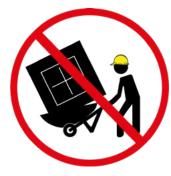
DO NOT USE A WHEELBARROW OR OTHER UNBALANCED EQUIPMENT TO MOVE UNIT
