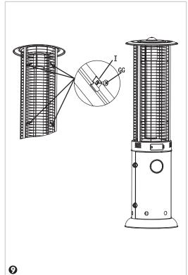
Attach the protection guard back with 4pcs M5x10 (GG).Complete.
