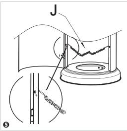
**5** Attach the Door (B) to the Back plate (C). Hook the Chain (J) into the holes of Back plate (C). 6 Attach the Up Cover (G) onto the Reflector (F) with 1pc M6x35 (EE) screw and M6 (BB) nut.
