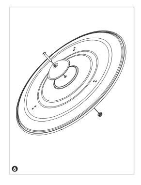
Unscrew the 6pcs preassembled M6x12 (FF) screws, attach the reflector onto the top,then fix them with M6x12 screws.
