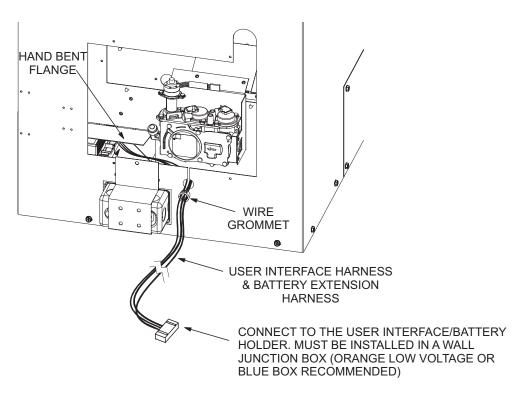
NOTE: OUTER ACCESS DOOR REMOVED. REPLACE AFTER ALL WIRE AND GAS CONNECTIONS HAVE BEEN MADE
