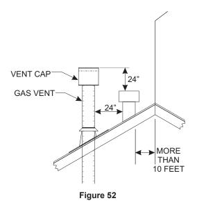
Note that for steep roof pitches, the vent height must be increased. In high wind conditions, nearby trees, adjoining roof lines, steep pitched roofs, and other similar factors can result in poor draft, or down-drafting. In these cases, increasing the vent height may solve this problem.
