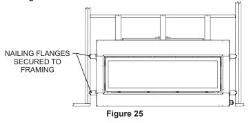
6. Attach three middle mount framing brackets to the top front edge of the fireplace. These brackets support the supplied non-combustible board above the fireplace. Preset depth to suit facing material (flush or 1/2in set back depths).
