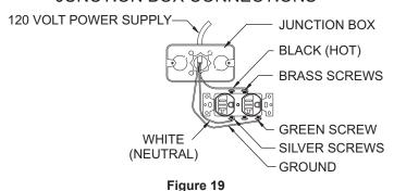
Install the receptacle into the junction box. Attach cover plate. After the wiring is completed to the junction box and receptacle, install the junction box to the lower right side of the fireplace as shown in **figure 20**. Insert the top flange of the retainer bracket into the slot on the fireplace. Rotate the junction box assembly downward, and secure with a screw below the junction box. **See Figure 20**.
