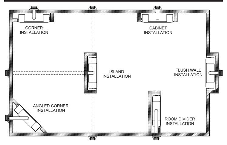
Note: Island and Room Divider installation is possible as long as the horizontal portion of the vent system does not exceed 20 feet with a minimum vertical run of 8 feet. See details in Venting Section.
