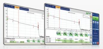
This improved linear view offers you the flexibility to display both the OTDR graph and its linear view without having to perform a toggle to analyze your fiber link.
