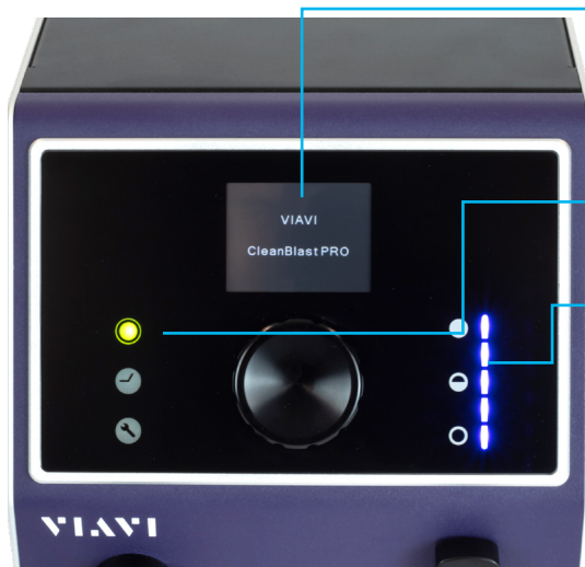
Figure 3: Front panel indicators and controls
