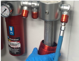
Unscrew lower section
