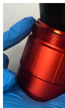
Grease and place lower section
