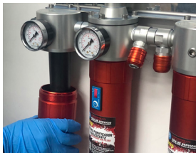
Unscrew lower section
