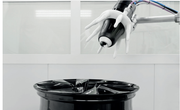
High-speed rotation atomizer with external charging
