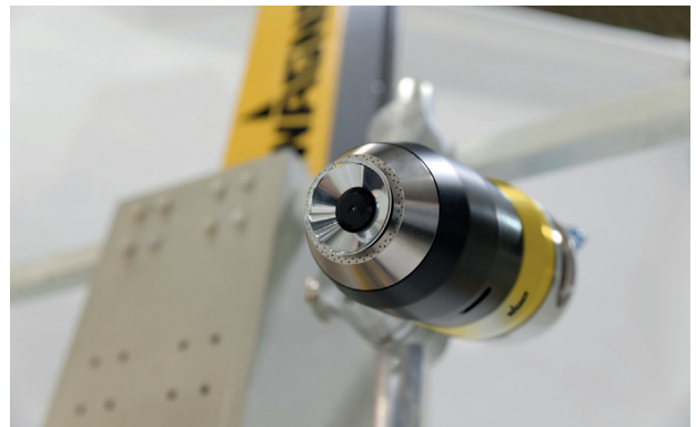
High-speed rotation atomizer with internal charging
