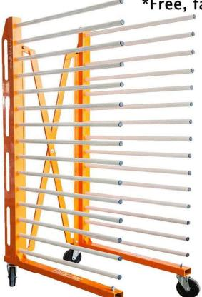
Our robust and expandable ProDryingRack EX stretches from 20" to almost 60" in width for the larger pieces of your project. Fifteen levels hold up to 60 lbs each. Round, 1" diameter, removable tubes of 30" lock into place with just a turn (no tools). If you need more than the 3" of usable space between the levels, just remove "levels" until you have the room you need.
