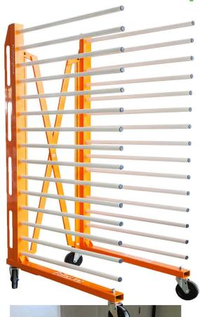
Our robust and expandable ProDryingRack EX stretches from 20" to almost 60" in width for the larger pieces of your project. Fifteen levels hold up to 60 lbs each. Round, 1" diameter, removable tubes of 30" lock into place with just a turn (no tools). If you need more than the 3" of usable space between the levels, just remove "levels" until you have the room you need.
