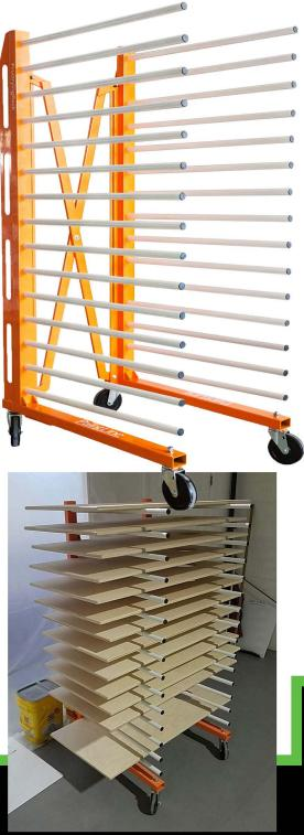
Our robust and expandable ProDryingRack EX stretches from 20" to almost 60" in width for the larger pieces of your project. Fifteen levels hold up to 60 lbs each. Round, 1" diameter, removable tubes of 30" lock into place with just a turn (no tools). If you need more than the 3" of usable space between the levels, just remove "levels" until you have the room you need.
