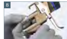
8 Install material flow control screw
