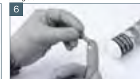
6 Grease and insert paint needle spring
