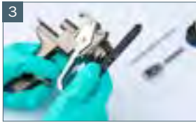
3 And finally, unscrew fluid tip with the ring spanner integrated in the universal spanner.
