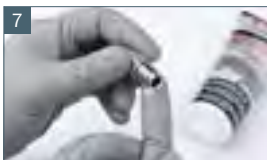
7 Grease thread of material flow control screw
