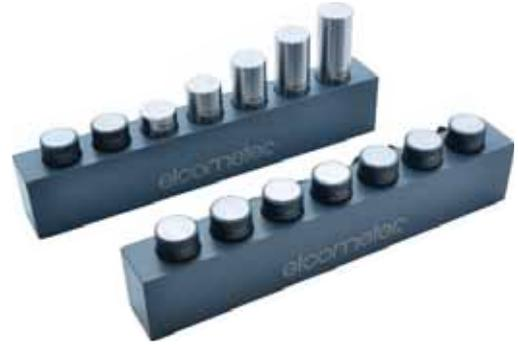
Calibration standard sets and individual standards are supplied complete with calibration certificate.
