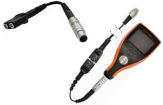
Simply plug the adaptor into the transducer connection point at the base of the gauge to connect any 'non-intelligent', dual element transducer and follow the on-screen instructions.
