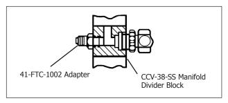
**Figure 3: Manifold Divider Block**
