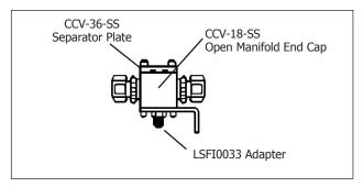
Figure 2: Two Valve Manifold Assembly
