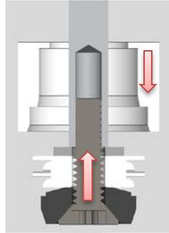
15. Place the assembled plunger shaft over the top of the pump cylinder. The seal tool will fit onto the top of the cylinder.
