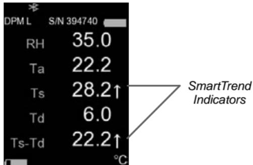
**Smart Trend™ Indicators ↑↓** - identify rising, falling or stable readings. The probe compares each measurement with recent values to provide the current direction of change.
