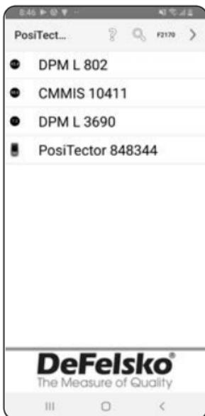
Once connected, the probe LED will flash every 3 seconds and the **PosiTector DPM L** will automatically download any previously logged datasets to the PosiTector App. The battery icon in the top left corner shows the battery level of the probe.
