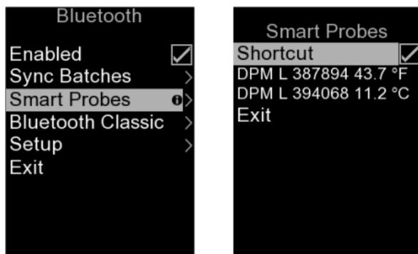
Checking the **Shortcut** box on the Smart Probes screen will enable access to the Smart Probes screen from the gage's main menu.
