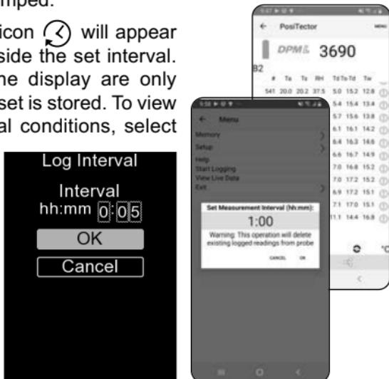
Logged datasets download automatically from the probe when connected to the PosiTector App or PosiTector Advanced instrument. Datasets are stored into a Batch (group). Each time a new Log is downloaded, all datasets are saved into a new batch.
