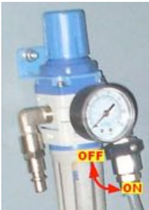
Pneumatic pump air supply valve
