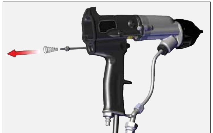
4. Remove air valve packing nut and packing.
