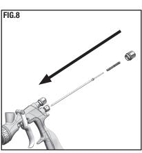
AIR CAP INDEX PIN (54-6184) INSTALLATION (OPTIONAL – 90° INCREMENTS INDEXING FEATURE)
