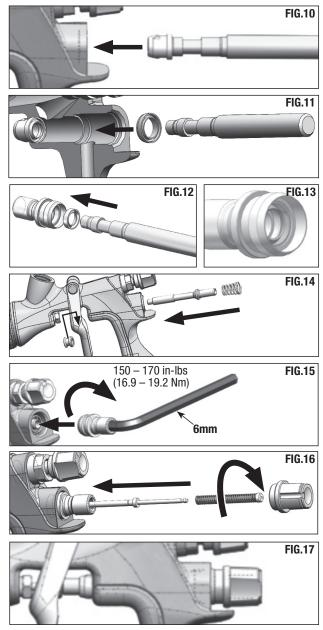
MAINTENANCE - FLUID NOZZLE AND BAFFLE REMOVAL AND INSTALLATION
