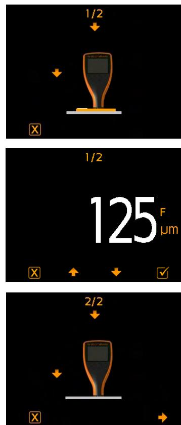
*Note: FNF gauges must be calibrated in both the ferrous and non-ferrous mode to ensure accuracy of readings.*
