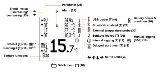
You can select which parameters to show on the reading screen and which of these should be displayed as the Main Reading - see page 28.
