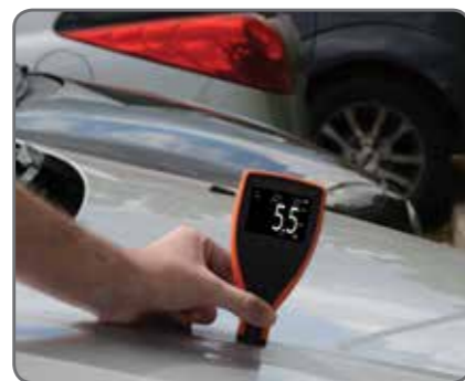
Measures on steel & aluminium body panels 2
