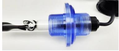
5 -Hand tighten the UV Cap Nut. Hold the UV Cap Nut and while keeping it straight 'GENTLY" twist the Quartz Sleeve. There should ne no movement - otherwise hand tighten a little more.
