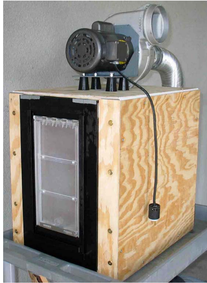
Figure 3.4. Experimental apparatus with a pet door unsealed for a total leakage test.
