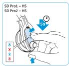
Push the Audio button in the direction "volume down" until the Headset LED goes off. The direction of the volume up/down function of the Audio button is changed. The headset switches to standby mode.
