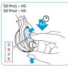
Push the Audio button in the direction "volume down" until the Headset LED goes off. The direction of the volume up/down function of the Audio button is changed. The headset switches to standby mode.
