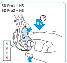
If pairing is not successful within 60 seconds, the headset switches back to standby mode.
