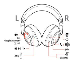
Power on/off Slide the switch  $\bigcirc$  to power on or off.
