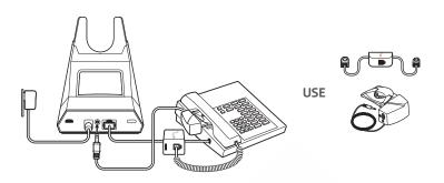
• Adjust the configuration switch on the bottom of the base to default **A**, which works for most phones. Use configuration **D** for Cisco phones.
